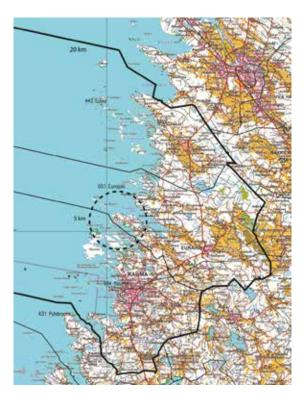
The precautionary action zone of the nuclear power plant extends to a distance of approximately 5 kilometres from the plant (indicated on the map with a dashed line). Restrictions related to land use apply in this zone.
